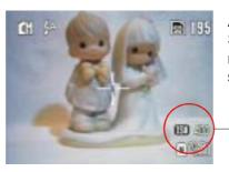
After you manually set the ISO Speed in the "Manual" capture mode, the ISO value will be shown on the LCD screen.
